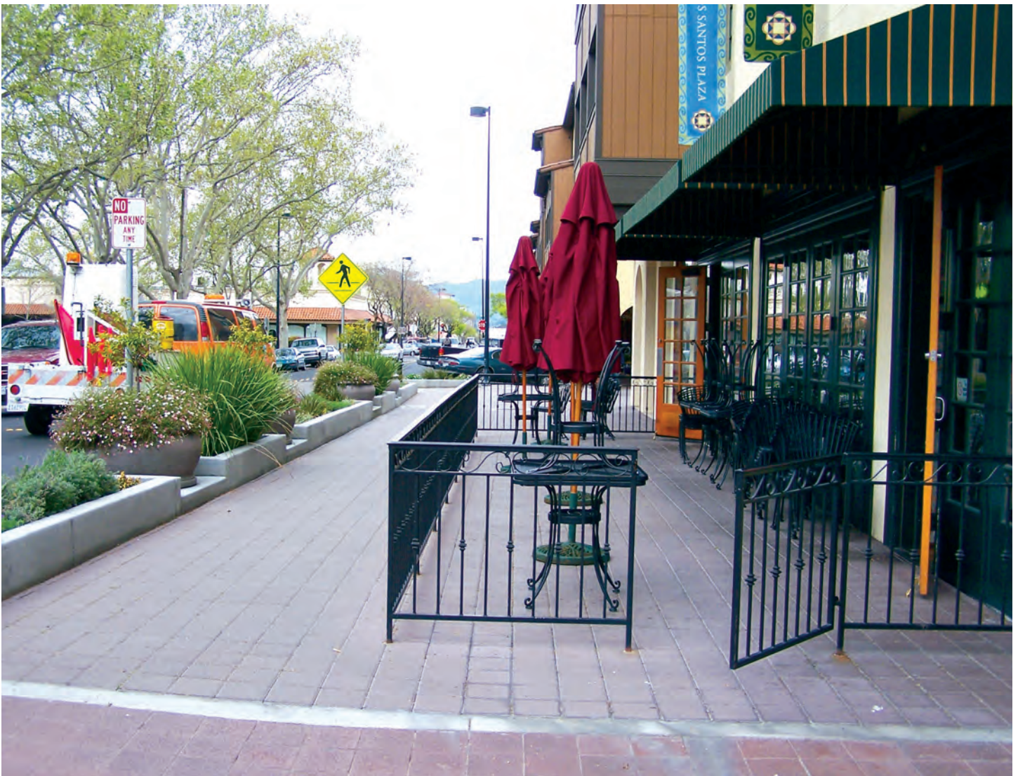
Territorial reinforcement in the form of fencing placed around the semi-private outdoor patio of a business.
