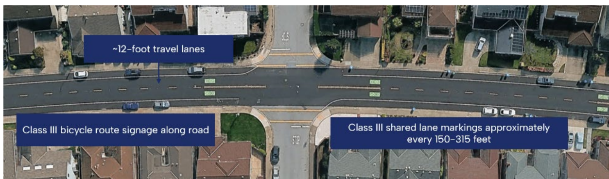
Marlin Avenue at Surfperch Street Class III Bike Route with 30 mph posted speed limit
