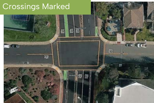
Catamaran Street at Shell Boulevard Visible (buffered) bike lane and standard crosswalk striping
