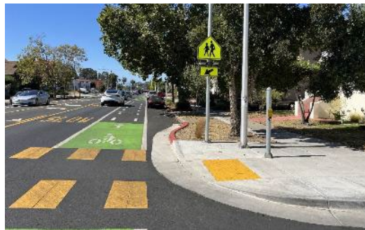
Rectangular rapid flashing beacon and High Visibility crosswalk Source: Federal Highway Administration.
